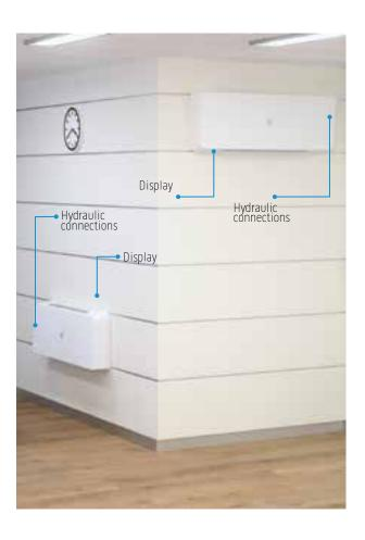
Bi2 Wall is the first hydronic terminal that can be installed as a split or as a console, by simply rotating the display on installation. In the split configuration, the water attachments are positioned on the right and the display is positioned on the left. In the console configuration, the water attachments are positioned on the left and the display is positioned on the right.
